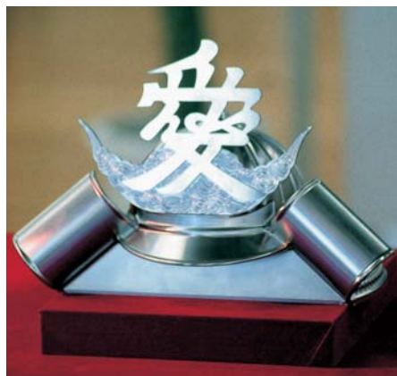
A helmet carved from a single material with a five-axis-control milling machine.
